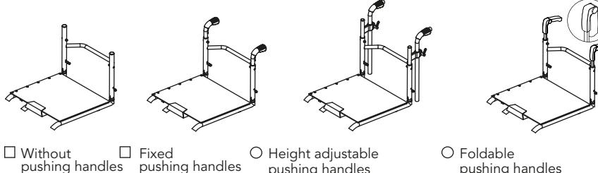
Without pushing handles  Fixed pushing handles  Height adjustable pushing handles  Foldable pushing handles
