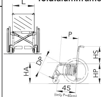
DP 19/21/23: only not detachable footrests & internally assembling of footplate DP 25/27/29/31: internally assembling of footplate
