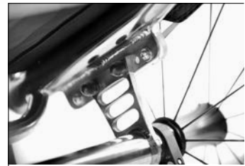
Baricentro fisso o regolabile. Fixed or adjustable centre of gravity.
