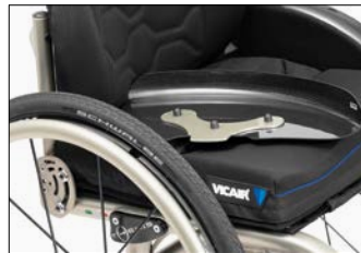
Spondine fisse o estraibili in carbonio. Fixed or removable carbon fibre clothes guards.
